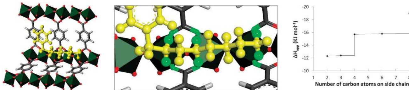
Fig. 10 Adsorption of alkylaromatics in MIL-47. The apparent adsorption enthalpy increases stepwise with the length of the alkyl chain due to an increasing number of hydrogen bonding contacts with the framework carboxylates. For n -octylbenzene (yellow), such interaction (green) can occur three times (V: gray octahedra; O: red; C: gray; H: white).
