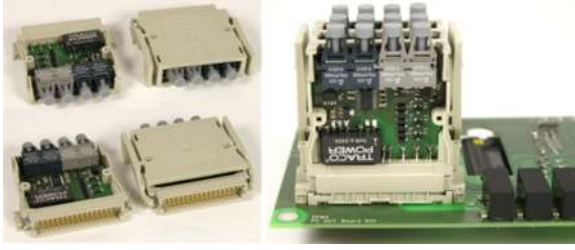
Fig. 7. Prototype of V_{CE\_ON} and V_F measurement circuit for the power cycling test.
