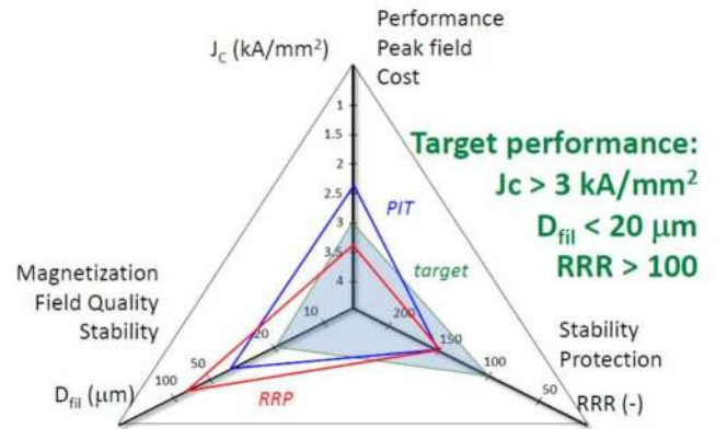
Fig. 2 The performance parameter space for Nb 3 Sn.
