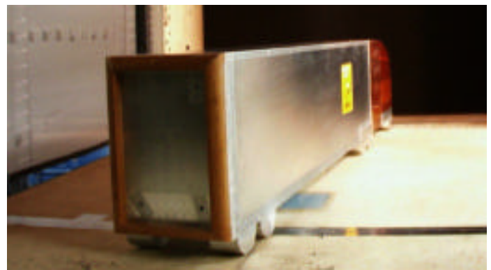
Figure 20 - Pneumatic Heavy Vehicle Model Installed Yawed (at Side-Wind Angle) in the GTRI Model Test Facility Subsonic Wind Tunnel
