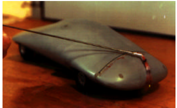
Figure 4 - Experimental Confirmation of Pneumatic Technology on a Streamlined Car; Aft View showing Blown Jet Turning
