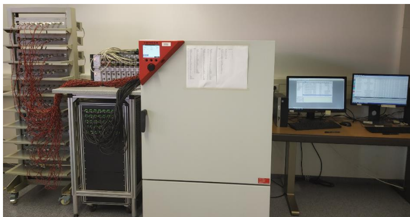
Figure 3.6 Photograph of Arbin BT-2000 battery test cyler and Binder climate chamber test systems used in this study.
