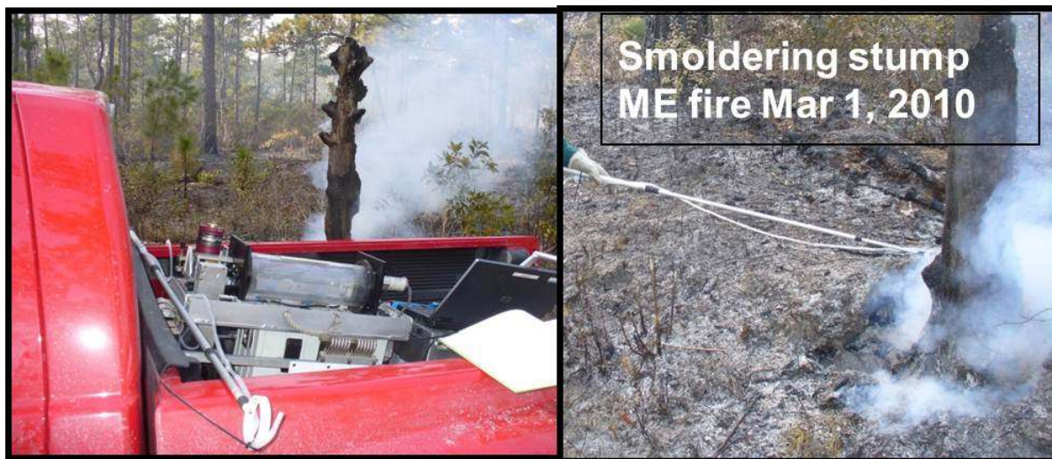
Figure 7.4 Photograph of the LaFTIR in back of pickup sampling burning stumps and burning live trees on 1 March 2010 at Camp Lejeune.
