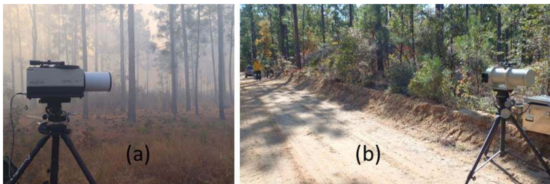
Figure 10.3 (a) Photograph of the OPAG-22 spectrometer and receiver telescope in the field. (b) Photograph of sender and receiver telescopes separated by an optical path of ~30 m.
