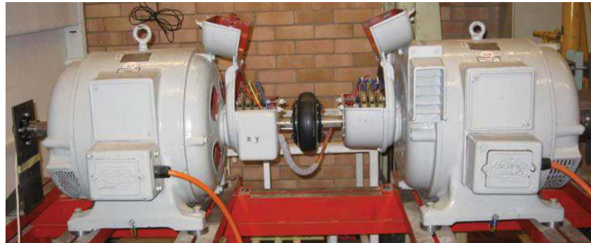
Fig. 2.8 Prototype of a 30 kW CBDFIG at UTS
