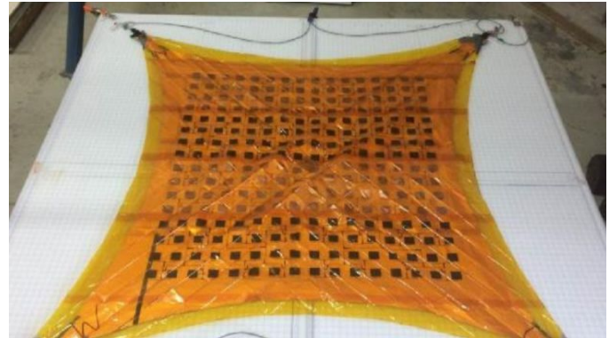
Fig. 13. S-band deployable membrane antenna after its first deployment [40].
