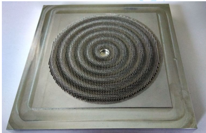
Fig. 7. Metal-only RHCP Ka-band metasurface antenna [15].
