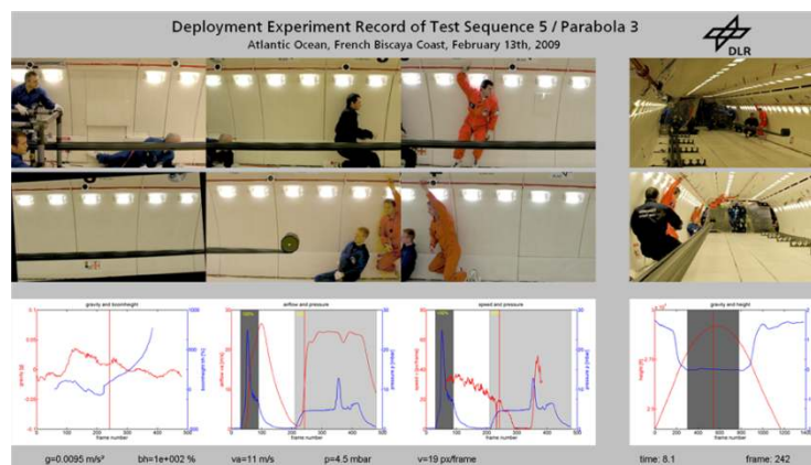
Fig. 18. Exemplary frame of a DLR parabolic flight campaign from 2009 used to verify different deployment control principles for DLR composite booms [19]
