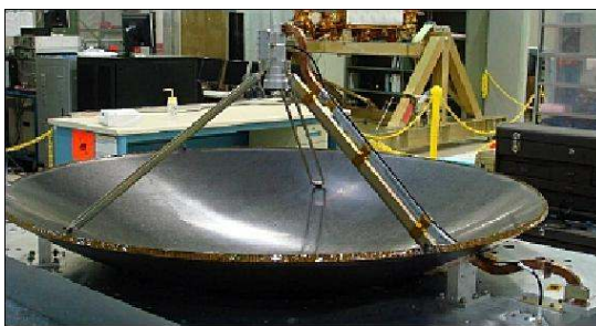
Fig. 1. Photo of the SRAL EM parabolic radar antenna of the European Sentinel 3 satellite (image credit: TAS, ESA)
