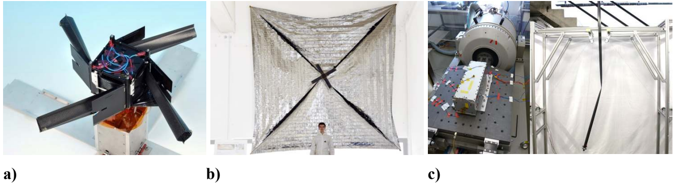
Fig. 17. DeorbitSail deployable structural subsystems: a) DLR developed small CFRP Booms & Deployment module, b) full size Qualification model of DeorbitSail at the DLR Space Structure Lab@ Uni, in Braunschweig, c) testing and qualifying CFRP booms and deployment module in DLR facilities (Source: DLR)
