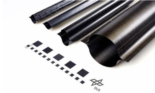
Fig. 9: DLR composite booms of different scale [Source: DLR]
