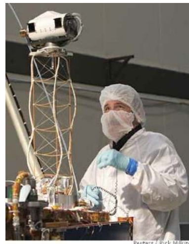
Fig. 6. Deployable stereo camera systems of Phoenix mars lander, (image credit: Lockheed Martin)
