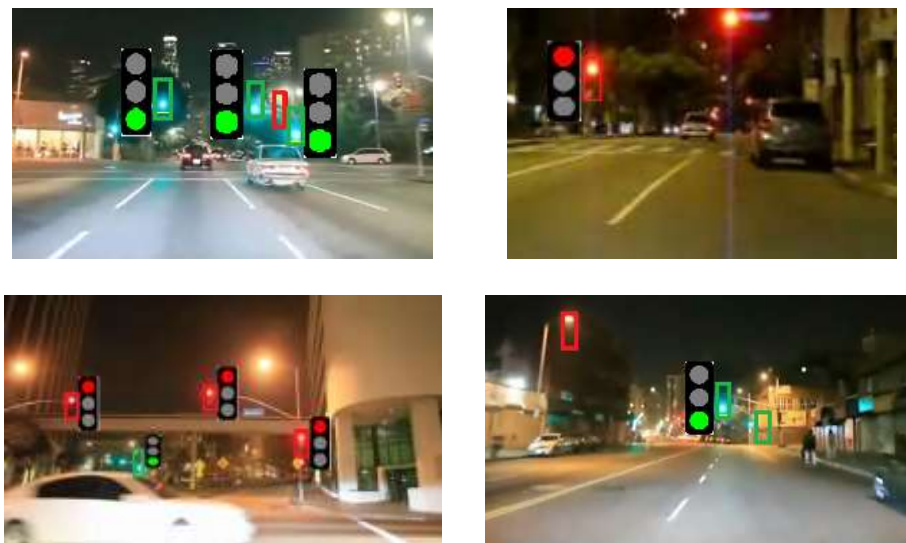
Figure 44 : TL detection results in urban night driving.
