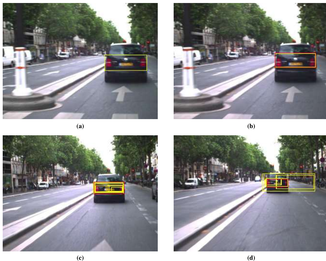
Figure 60: Example of Kalman tracking in the LARA video dataset. The vehicle detections are shown in yellow rectangles while the red rectangles denote the target being tracked.
