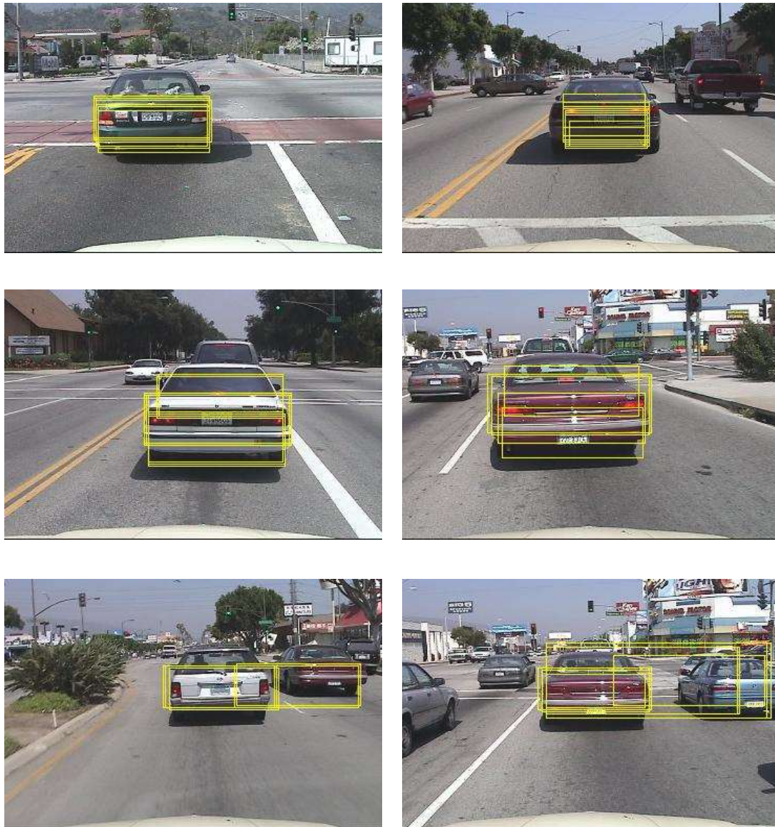
Figure 58: Multiple ROIs generated by the HV module.
