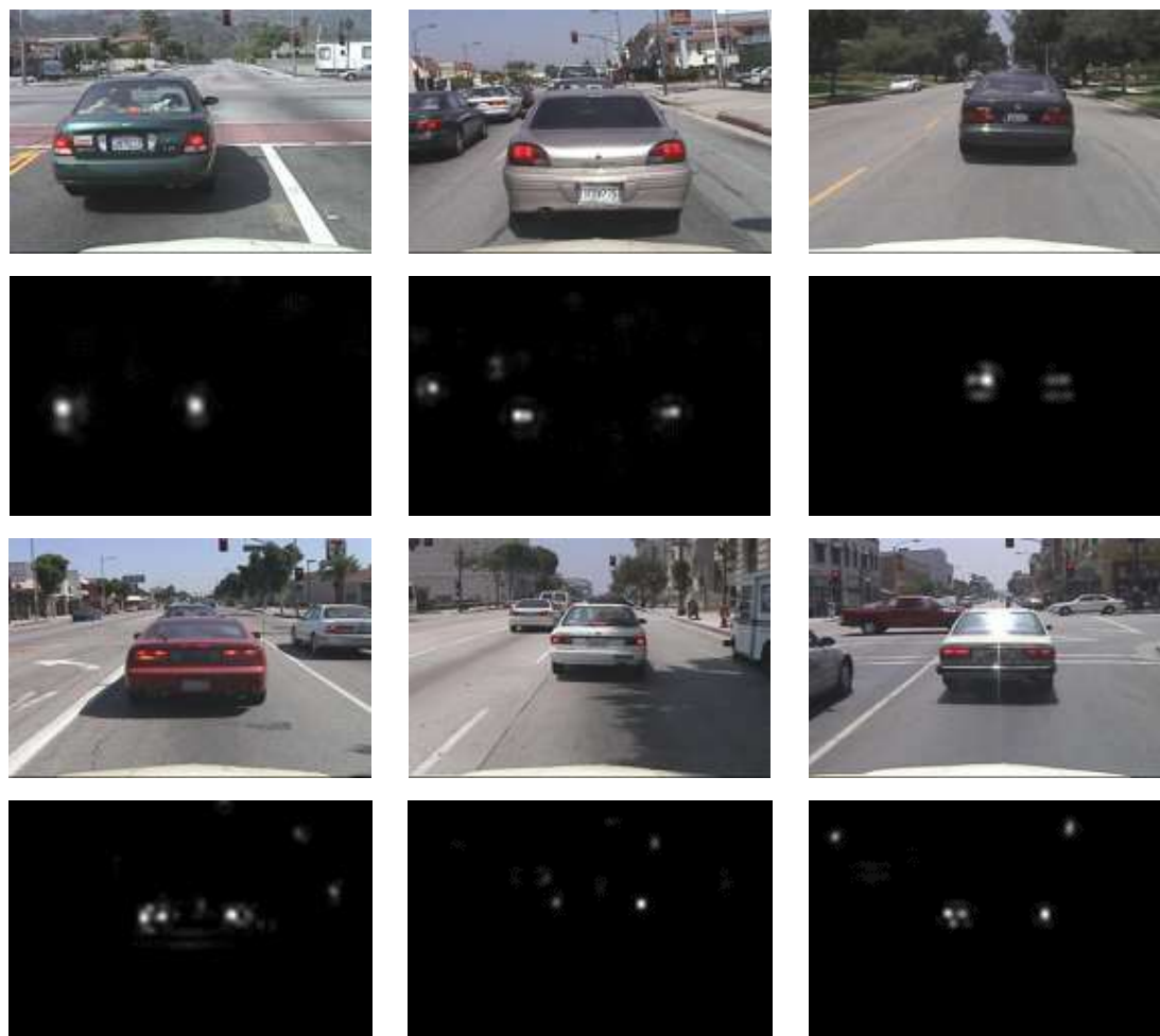
Figure 54: Various examples of FRST based detection of preceding vehicle rear lights. The original images appear in odd rows and the respective FRST results in even rows. The results have been estimated for one radius (8 pixels for top rows and 6 pixels for bottom rows).
