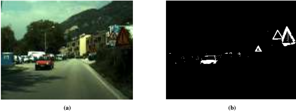
Figure 14 : (a) Original image and (b) Otsu's thresholding on channel a* of the image.
