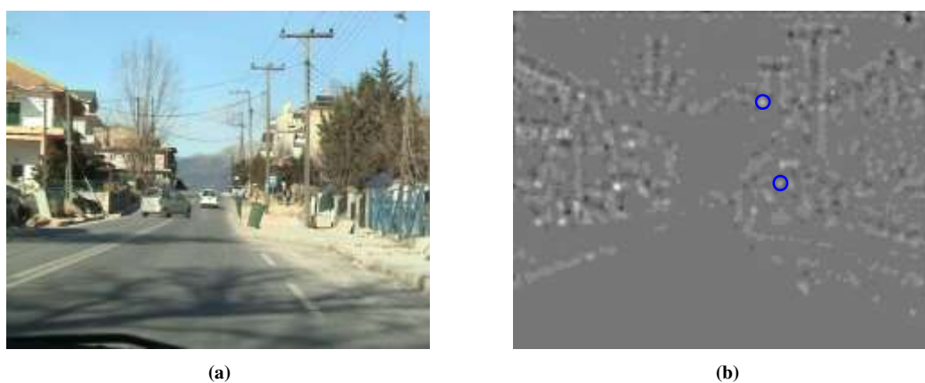
Figure 25: (a) Original image with a blue rectangular TS present and (b) detected FRST centers from all 4 channels for radii of size n = 5 , n = 8 and n = 11 . Blue circles denote the two most prominent blue results.
