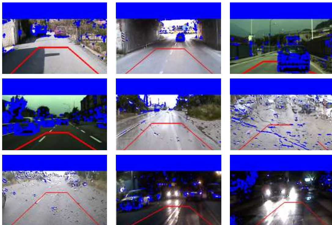
Figure 65 : Non-road (blue pixels) and road (red pixels) seeds using the proposed method in various conditions.
