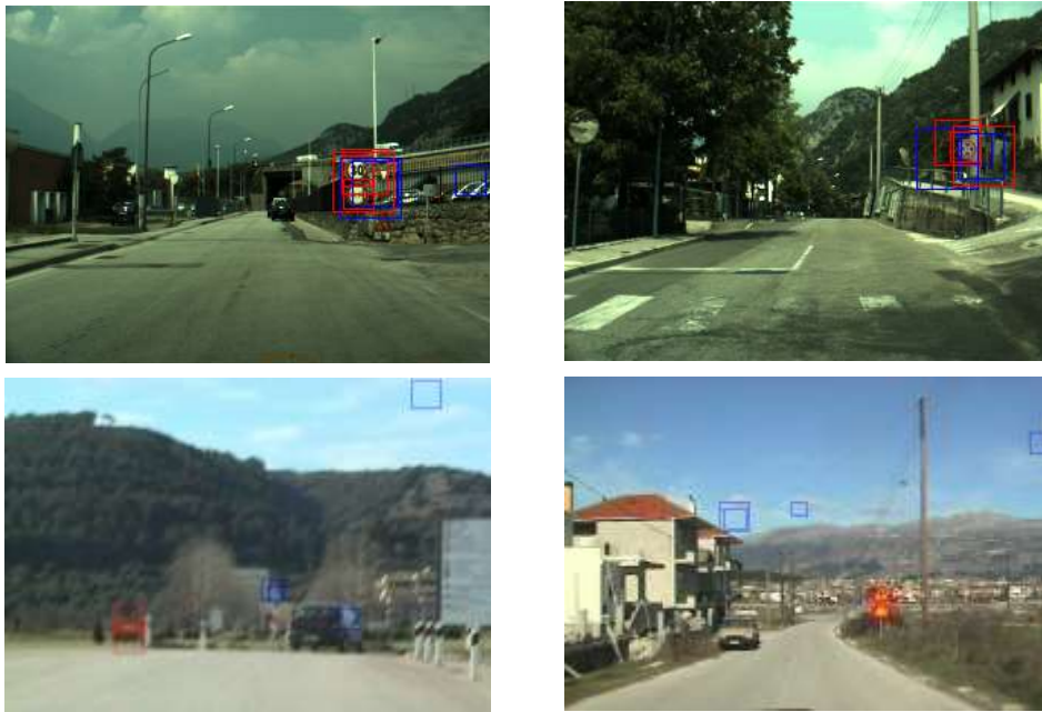
Figure 30 : Typical TSD examples for a single frame using radii in {10, 15, 20}.
