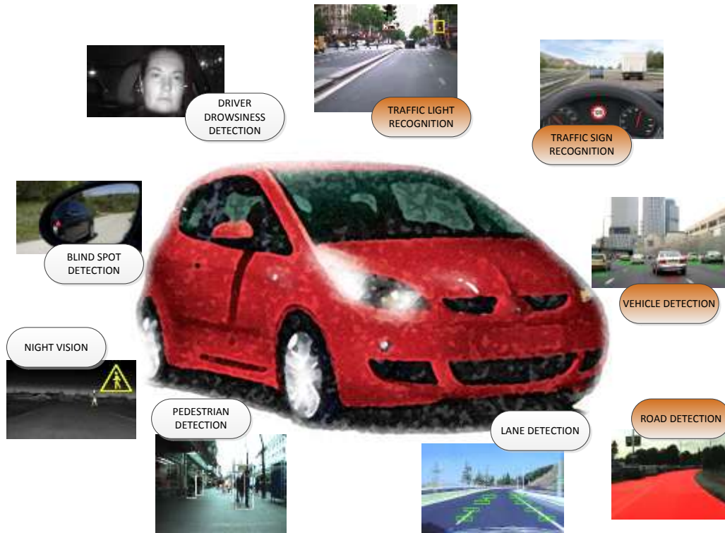
Figure 9 : Structure of a complete, entirely vision-based ADAS. The highlighted systems are covered in this thesis.
