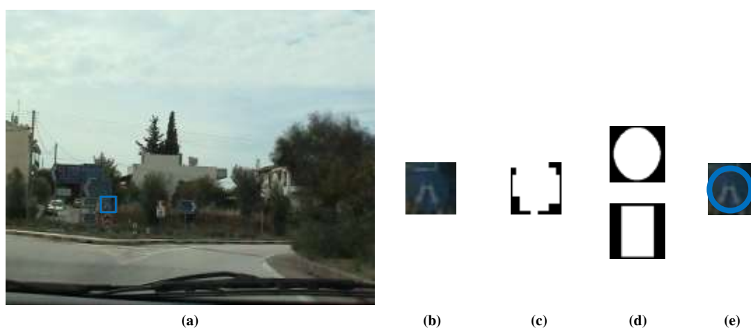
Figure 27: (a) The original image with the results of non-maxima suppression for the total FRST, (b) cropped candidate TSs, (c) binarized TSs, (d) shape templates and (e) classified shape overlaid on candidate.
