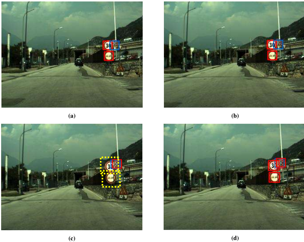
Figure 28: (a) First frame and detected TS candidates of 10px radial, (b) second frame and detected TS candidates of 10px radial, (c) third frame and detected TS candidates of 10px radial, (d) third frame and detected TS candidates of 10px radial, plus detected TS candidates of 11px radial around the areas of previously detected TS candidates (yellow rectangles in (d)).
