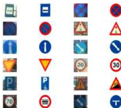
Figure 33 : Examples of correct (top four rows) and incorrect (bottom two rows) classifications using the frame-by-frame method.
