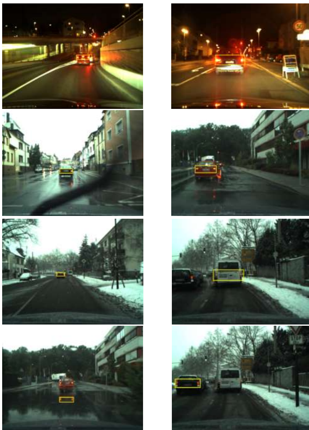
Figure 61: Examples of vehicle detections from the proposed system in adverse conditions. Top row: night driving. Second row: driving in the rain. Third row: driving in snow. Fourth row: Typical false positive examples.
