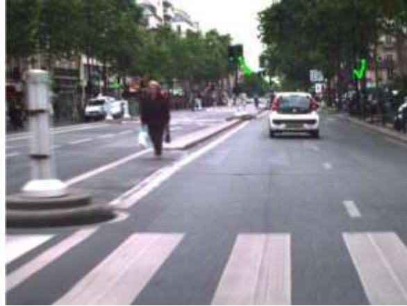
Figure 40 : Spatiotemporal persistency check. Notice the trails left by the centers of two green TLs.
