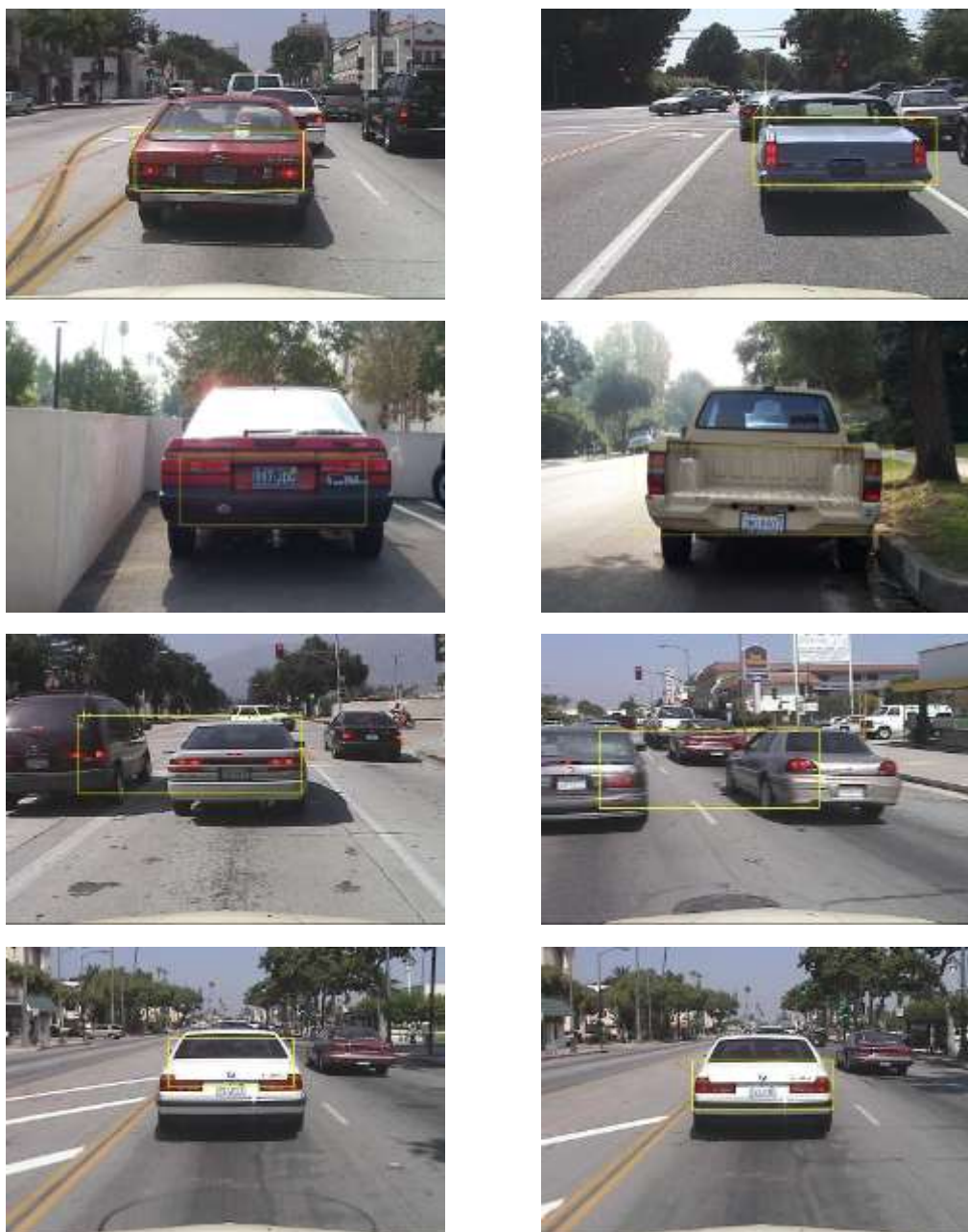
Figure 59: Successful detection results from Caltech 2001 (first row) and Caltech 1999 (second row). Two false positive results between two closely moving vehicles are shown in the third row. The problem of spatial inconsistency of the detection result in consecutive frames is demonstrated in the bottom row.
