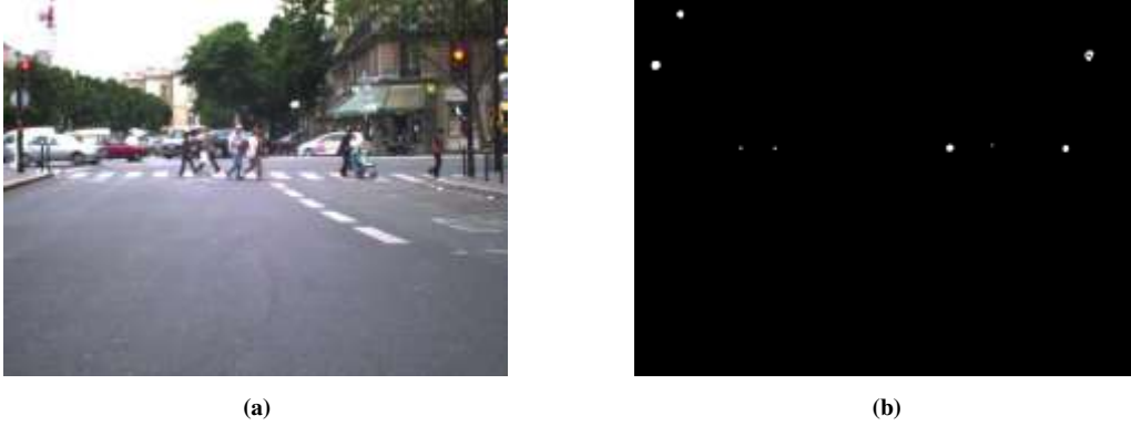
Figure 15 : (a) Original image and (b) result of Otsu's thresholding on the FRST of channel a^* .
