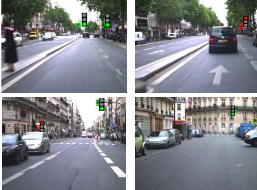
Figure 42 : TL detection results in daytime driving. A false positive red color TL example is show in the bottom left image and a false negative is shown in the bottom right.
