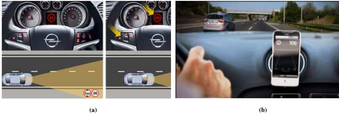
Figure 4: (a) Opel Eye system uses a camera to recognize speed signs and warn the driver. (b) Mobileye's traffic sign recognition system. It recognizes speed signs and warns the driver if speed limit is exceeded.
