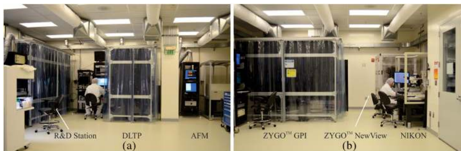
Fig. 3 Lab arrangement and metrology instrumentation in the ALS XROL cleanroom: (a) R&D Station, developmental long trace profiler (DLTP), and atomic force microscope, Veeco™ Dimension-3100, and (b) 6-in. aperture Fizeau interferometer, ZYGO™ GPI, interferometric microscope, ZYGO™ NewView-7300, and an optical microscope, NIKON™ MM-800/L. The second interferometric microscope, MicroMap™-570, is placed on the ZYGO™ GPI optical table. The NOM-like gantry system and the LTP-II with granite table are not depicted here.
