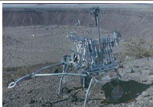
Figure B.3-5. The Apollo 14 astronauts used this prototype of the MET during their geological and lunar surface simulation training in the Pinacate volcanic area of northwestern Sonora, Mexico. (NASA photo S70-29505).
