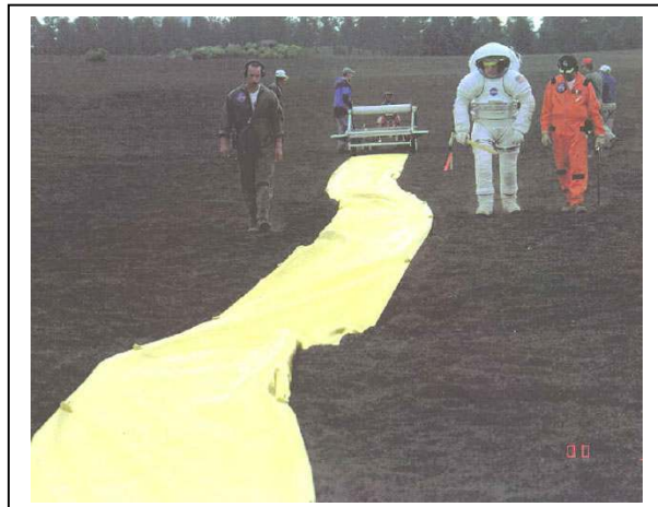
Figure C.4-9. Testing the deployment of a solar array at Cinder Lake, Arizona. (NASA photo)
