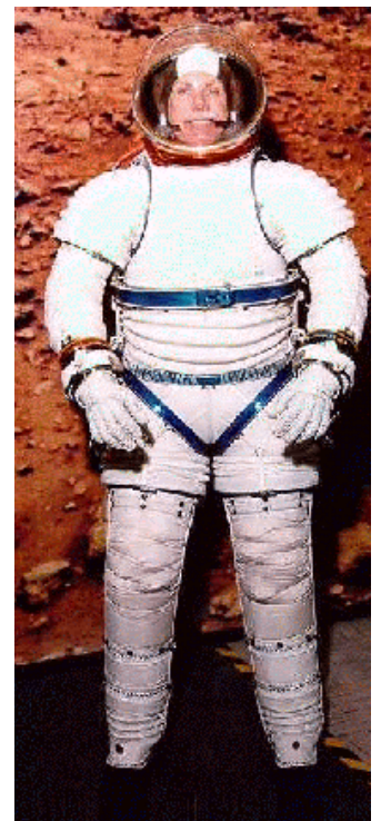
Figure C.1-14. The I-1 experimental EVA suit developed by the ILC Corporation.
