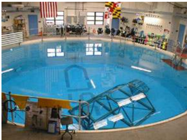
Figure C.4-5. The deck area of the NBRF. In the tank is a mock-up of a section of the ISS main truss. (UMD photo)
