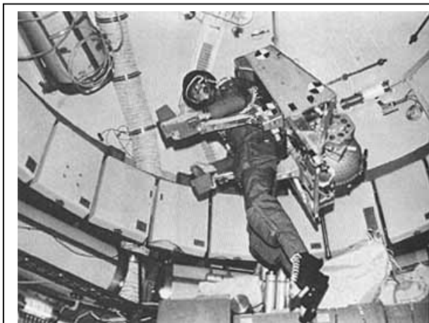
Figure B.3-3. A Skylab 3 onboard photo shows astronaut Jack Lousma as he flew the M509 AMU in the forward dome of Skylab while in Earth orbit.
