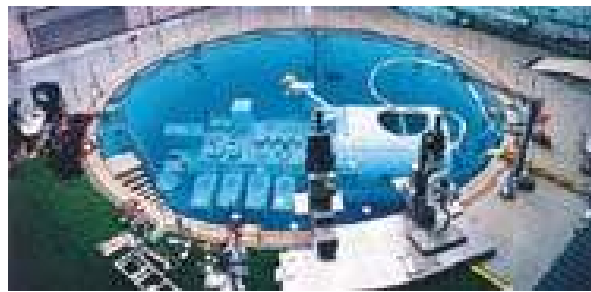
Figure C.4-4. The NASDA neutral buoyancy facility with a full-scale mock-up of the Kibo module destined for the International Space Station. (NASDA photo)
