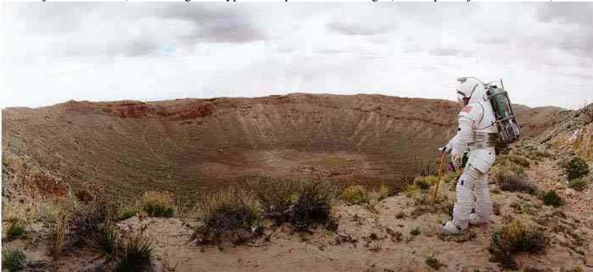
A test subject in the Mark III experimental surface EVA suit at Meteor Crater, Arizona
