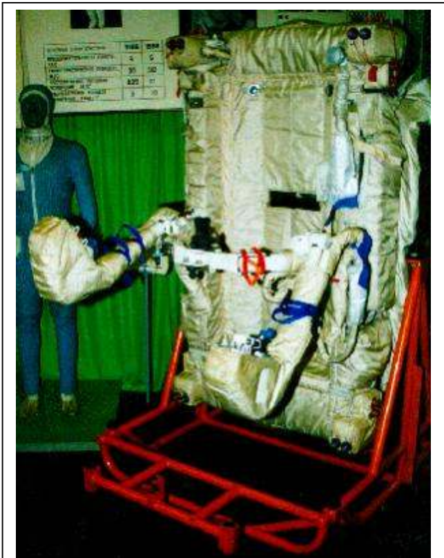
Figure B.1-10. The SPK maneuvering unit, designed for use with the Orlan-DMA suit.
