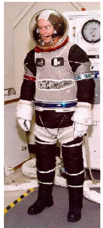
Figure C.1-12. The D-1 (S1035X) experimental suit developed by the David-Clark Company.
