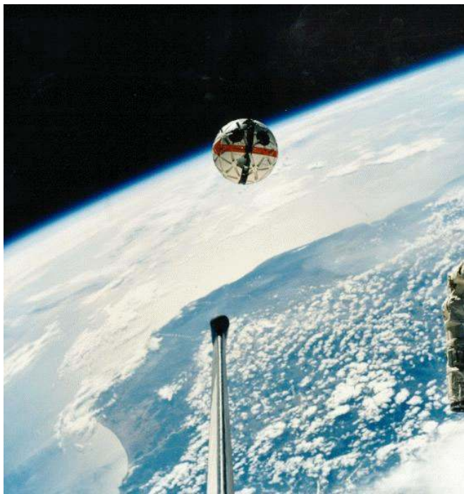
Figure C.2-4. AERCam Sprint during its orbital flight demonstration on STS-87. (NASA image STS087-752-035)
