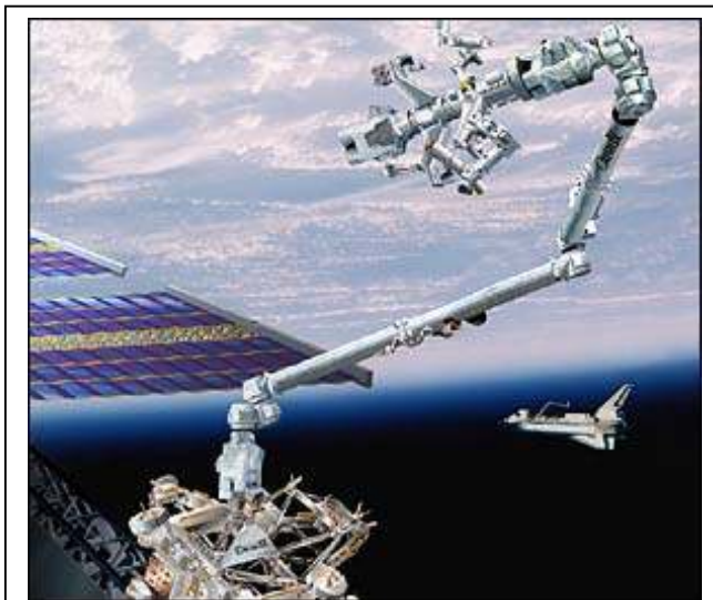
Figure C.2-2. A general view of the Mobile Servicing System, including the Mobile Base System and the Special Purpose Dexterous Manipulator. (Image courtesy of the Canadian Space Agency)
