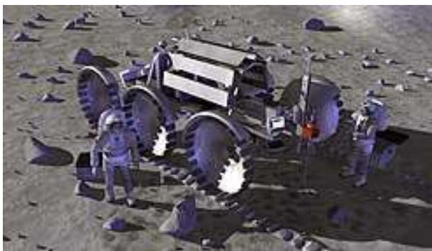
Figure E-6. An unpressurized rover equipped with a small drill powered by the rover's power plant and energy supply. (NASA image)
