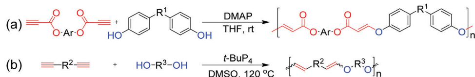
Fig. 9 Hydroxyl-yne click polymerizations: (a) DMAP-catalyzed aromatic hydroxyl (phenol)-yne click polymerization and (b) superbases t -BuP 4 -catalyzed aliphatic hydroxyl-yne click polymerization.
