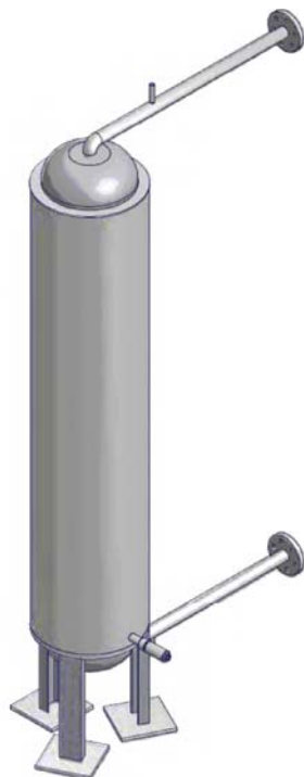
Figure 4: \text{NaNO}_3 PCM Storage Test Module
