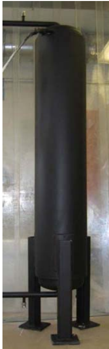
Figure 4: \text{NaNO}_3 PCM Storage Test Module
