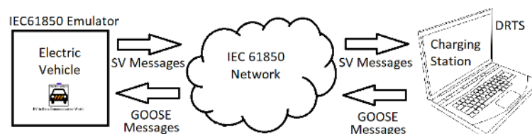
Figure 22. HIL test set-up for model validation.
