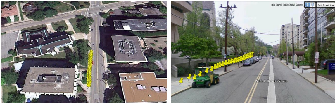
Figure 5.29. Geo-positioning results by using visual odometry, top view (left) and street view (right)
