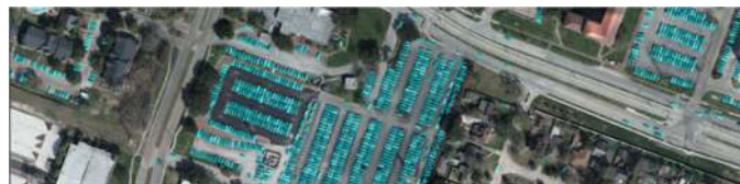
Fig. 9. Detail of pixel-wise car segmentation in VHR RGB data. The detected cars are highlighted in blue.
