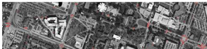
Fig. 8. Detail of crosswalk detection in VHR RGB data. The detected crosswalks are highlighted in red.
