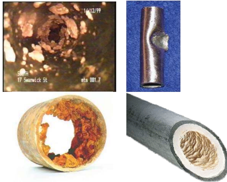
Figure 8.2 Blockages in a Pipeline System
