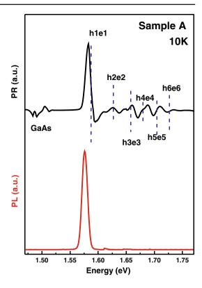
sample structure obtained after the growth process. Based on energy of optical transitions and results of theoretical calculations, we can get the information about positions of the electron and hole levels in the investigated structure. In this way we can verify the assumed growth parameters (width and the contents of the layers), by analysis of the estimated quantum fine structure.
