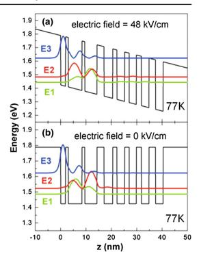
situation, E2–E1 distance should be around  $\sim$ 30 meV (GaAs optical phonon energy), which provides tunneling the electron from E2 to E1 and further through injector part to the next cascade.
