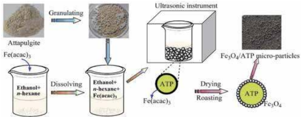
Figure 11. Schematic of preparing Fe 3 O 4 /ATP catalyst [24].
