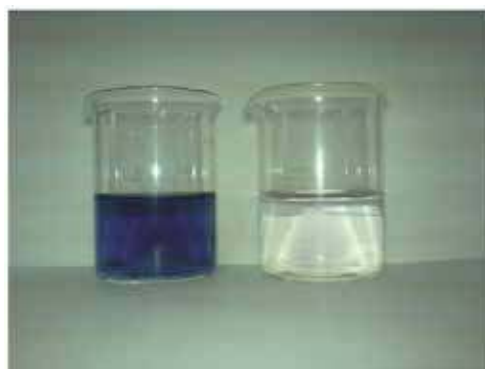
Figure 16. Samples collected during a typical experiment before (left) and after (right) photocatalytic treatment.
