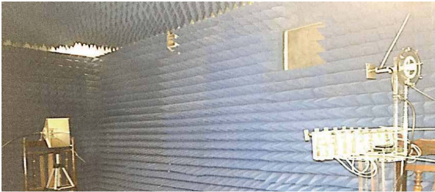
Figure 31. Array antenna measurement in anechoic chamber.
