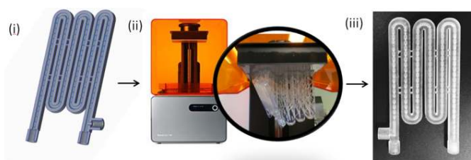
Figure 1: The stages of AM fabrication of a mini-OBR device. (i) A CAD model was designed to meet requirements. (ii) The reactor device was fabricated using Form2 SLA printer. (iii) The reactor was polished, cleaned and extensively flushed with IPA to remove residual uncured resin.
