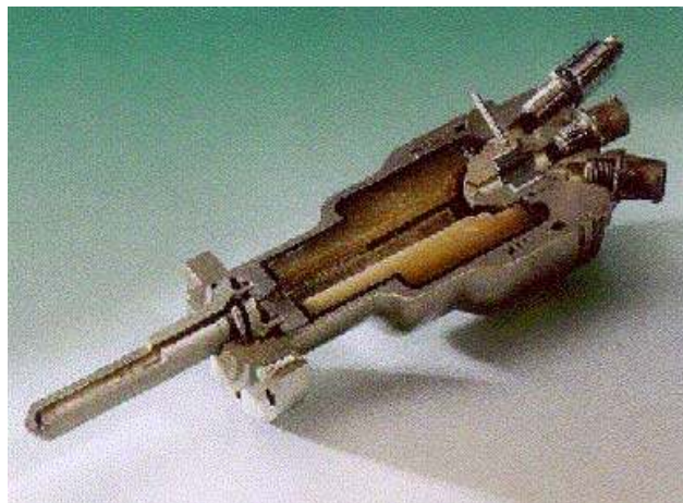
Figure 10: Pyrotechnic ignition system of the Vulcain engine
