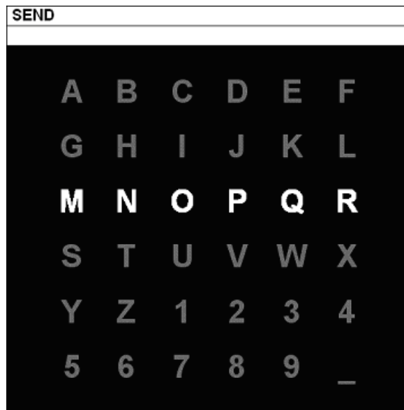
Figure 1: P300 response. P300 response is an event related potential which is triggered by the infrequent events in an oddball paradigm.
