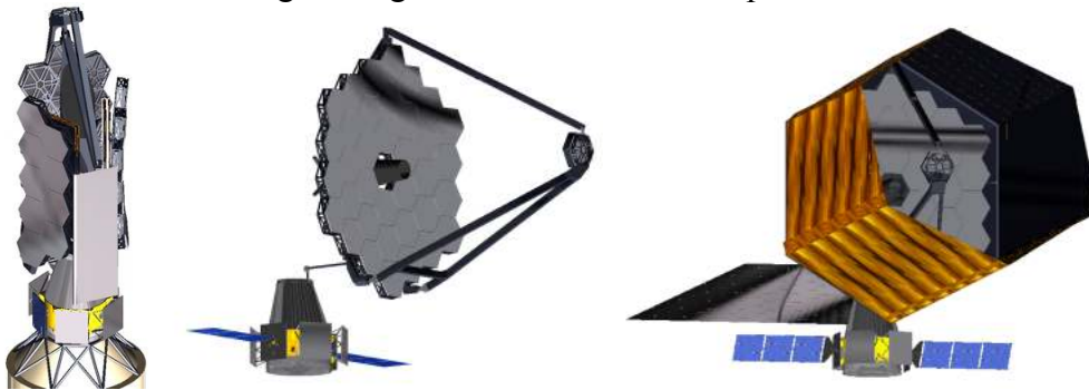
Figure 7: (Left) Stowed 16.8-meter OTA. (Center) 16.8-m ATLAST deployed but the sunshade and “kite tail” (to mitigate solar torque) are not shown. (Right) 16.8-m shown with sunshade, “kite tail,” and arm-mounted OTA.
