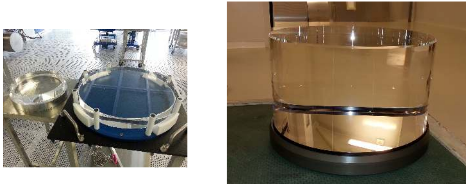
Figure 4. LEFT: Power Recycling substrate (35 cm in diameter, left) beside the large Beam Splitter of 55 cm. RIGHT: a test mass.
