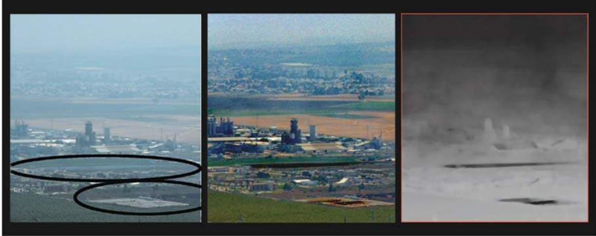
Figure 2. Naive dehazing when specular objects exist in the field of view. [Left] The best-polarized image of the scene, I_{\min} . Note the specular objects (water reservoir, nylon sheets).[Middle] In the naively dehazed image, the color has distorted to black in the specular objects area. [Right] The range map shows anomalies in those areas as well. For high resolution color images, link to Ref. 11
