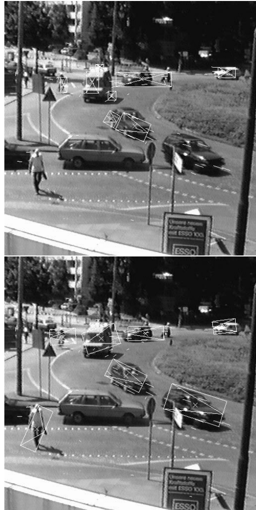
Figure 6: Frame 140. Top: direct approach fragments object bounding boxes (compare with next two frames). Bottom: belief revision approach captures most moving objects consistently in successive frames.
