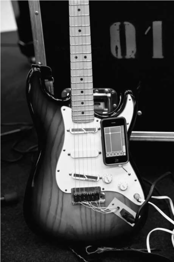
Figure 5. iPhone control interface mounted on the Feedback Resonance Guitar.
