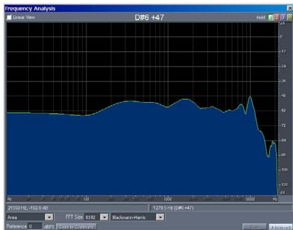
Fig. 16 – measured frequency response of the artificial mouth system
