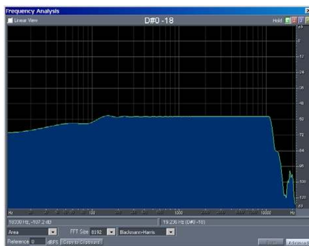
Fig. 19 – measured frequency response of the artificial mouth system after equalization
