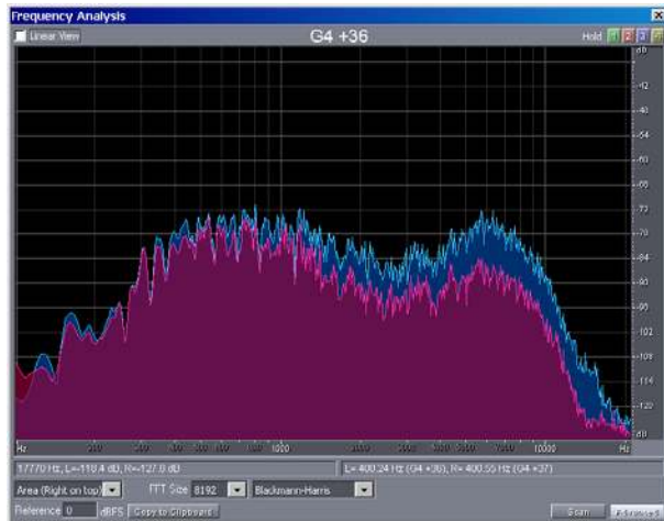
Fig. 36 – spectrum of single sweep of 50s (above) versus 50 sweeps of 1s (below)
