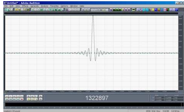
Fig. 9 – reduced pre-ringing artifact without fade-out
