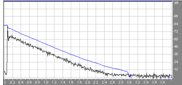
Fig. 31 – octave-band filtered IR with pulsive event removed with FFT filter
