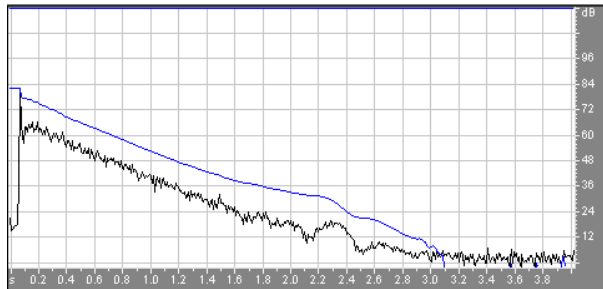
Fig. 25 – octave-band filtered IR with silenced pulsed event
