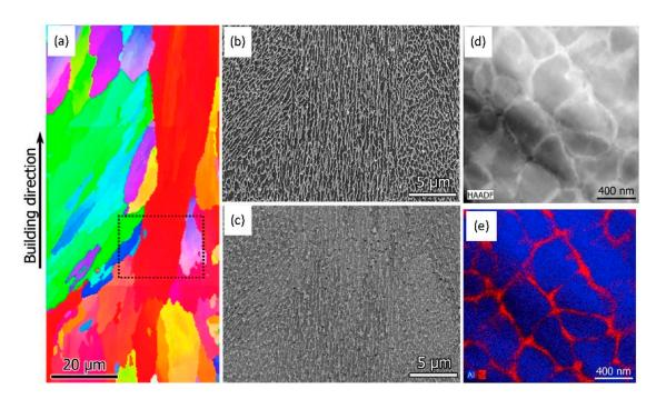
**Figure 17.** The (a) EBSD image depicts the AlSi10Mg alloy grain structure obtained by SLM with columnar cells developing perpendicular to the build direction, (b,c) SEM images show the microstructure in the dashed region and the grain structure using a secondary electron detector, and a backscatter electron detector, respectively. As-built SLM AlSi10Mg cells' STEM images and associated Al-Si EDX maps are displayed in (d,e) [207].
