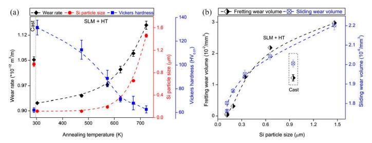
**Figure 14.** (a) Influence of heat treatment process on the hardness and wear of AlSi12 alloy formed by SLM approach, (b) tribological behavior of the materials formed by SLM approach comparable to cast counterpart [145].
