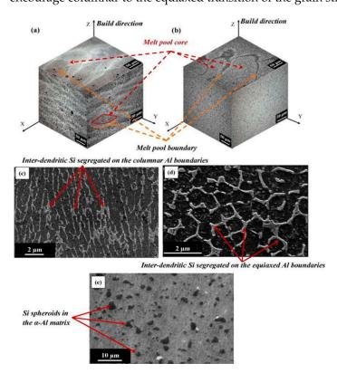
**Figure 16.** The microstructure of SLM AlSi10Mg is shown in isometric views in the following order: (a) as-built, (b) after heat treatment; (c,d) elongated  $\alpha$ -Al and equiaxed  $\alpha$ -Al grains as seen on the XY plane in the as-built material and (e) Si spheroids in the  $\alpha$ -Al matrix after T6 heat treatment [192].
