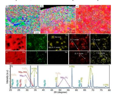
**Figure 4.** EBSD image shows equiaxed, fine, and random grain representation in (**a**) bulk LPBF-WE43, (**b**) last melt pool corresponds to basal- orientated, large, and irregular shape grains, (**c**) basal-orientated, large, irregular shape grains in the bulk sample, (**d**,**e**) EDS image at different magnification for same materials, and (**f**) XRD image depicted intermetallic and oxygen-rich elements in WE43 alloy [27,33,56].
