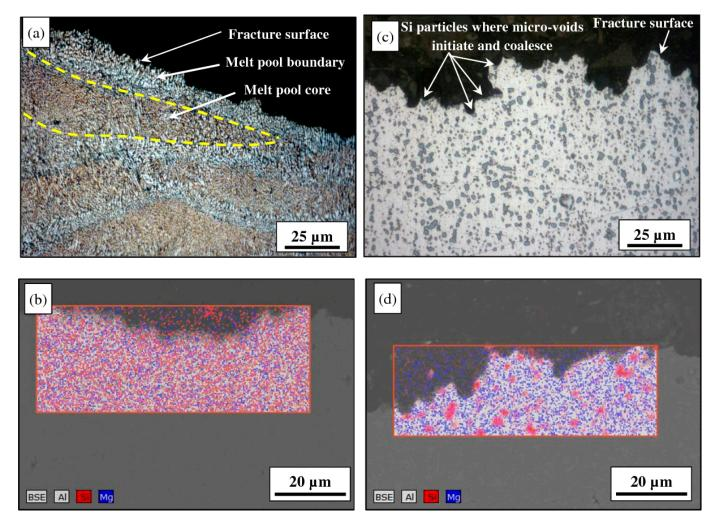
**Figure 11.** Tensile fracture of AlSi10Mg alloy formed by SLM approach oriented cross-sectionally comparing (**a**) as-built sample in the horizontal direction with EDS mapping (**c**), the heat-treated specimen (**b**,**d**). The fracture surface of an as-SLM specimen is oriented in the horizontal direction [161].
