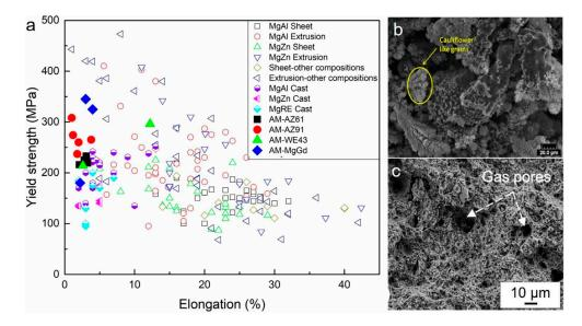
**Figure 5.** (a) Tensile characterization of additively manufactured Mg-based material via LPBF approach against wrought and cast alloys, (b,c) Fractured surface of (b) Mg-9Al alloy and (c) WE43 alloy [27,46,54].
