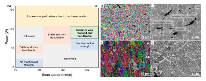
**Figure 3. (A)** Processing parameters of laser-based powder approach, **(B) (a–c)** depicted EBSD orientation, **(b–d)** SEM characterization of AZ91 alloy formed by laser powder bed fusion [27].
