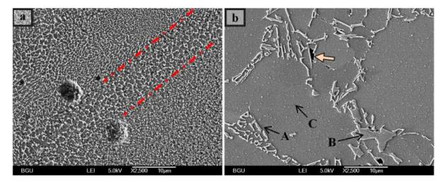
**Figure 15.** SEM image depicted AlSi10Mg microstructure formed by (a) SLM, and (b) casting. The arrows in (b) point to (A) Al-Si eutectic, (B) Si dispersed in Al matrix, and (C) Fe-containing intermetallic phases [191].
