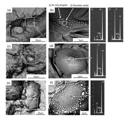
**Figure 13.** Backscattered electron images for oxide particles at the boundary between defect area and crack propagation region. An overview at lower magnification is given in (**a**,**c**,**e**), and detailed surface morphology in (**b**,**d**,**f**). Typical EDX spectra at right show the presence of Al and Mg in oxide particles [193].
