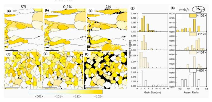
**Figure 20.** (**a**–**f**) Mapping distribution of grain orientation, (**g**) grain size, and (**h**) grain aspect ratio of SLM Al–Mn-Sc alloys [252].
