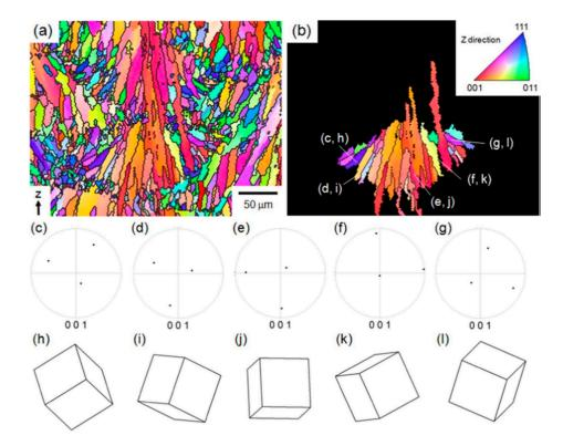
**Figure 18.** (a–l) Inverse pole figure orientation map displaying the elongated grain structure's predominately {1 0 0} orientation along the build direction. Additionally, the orientation map reveals a finer grain structure at the melt's sides and top, but there is no clear dominating orientation [208,211].
