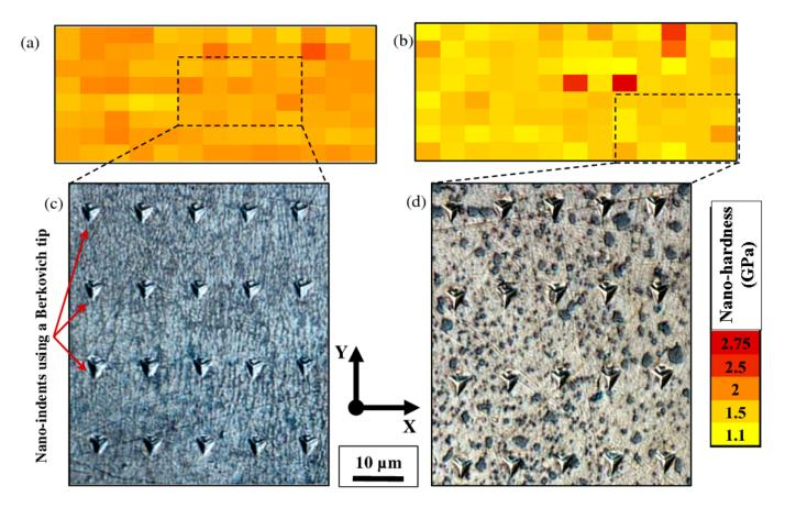
**Figure 7.** Nano-hardness image of an AlSi10Mg alloy fabricated on cast AlSi12 substrate depicted the homogeneity in the SLM material vs the non-uniform profile in the related part; Comparison in the nano-hardness of (a,c) the as-built material, and (b,d) the heat-treated material [161].
