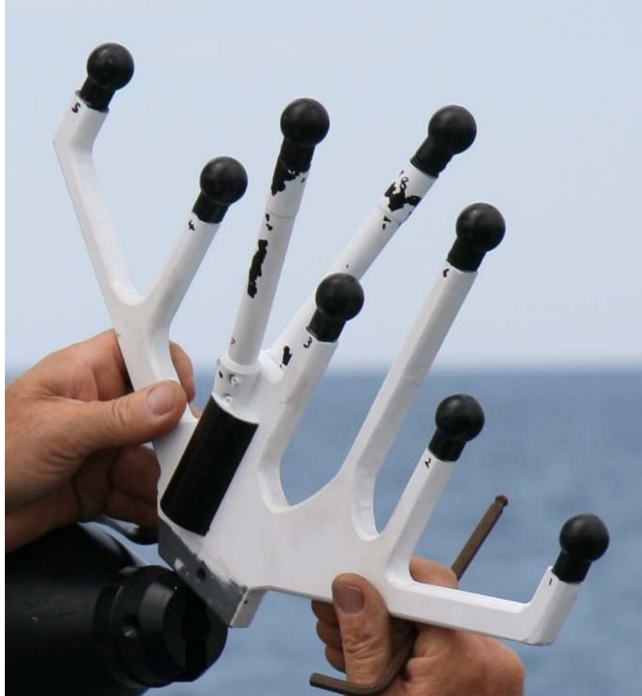
Figure 6.6: The passive acoustic array consisted of tetrahedral and line sub arrays. This was mounted to the nose of the eFolaga AUV.
