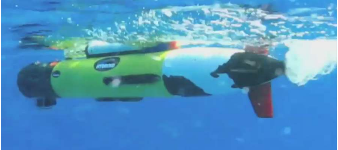
Figure 4.7: Photo of the REMUS-100 AUV as it is deployed from the small boat. Bubbles are likely due to air entrainment at the surface.
