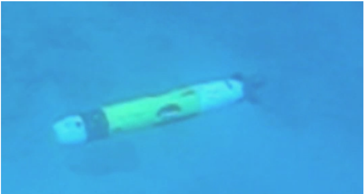
Figure 4.8: Photo of the REMUS-100 AUV as it moves several meters below the surface. Despite the lack of clarity in this photo, note the lack of bubbles behind the propeller. This suggests that the propeller is not cavitating in these conditions, which affects the amount of broadband radiated noise.
