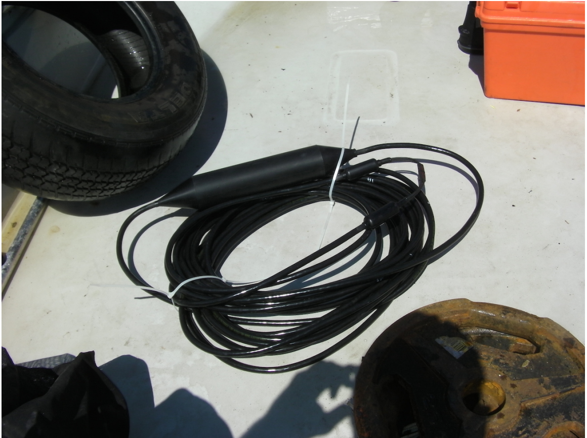
Figure 4.6: Photo of the synchronizer that fed a known electrical waveform to the first channel of each array, allowing the arrays to be time synchronized in post-processing.
