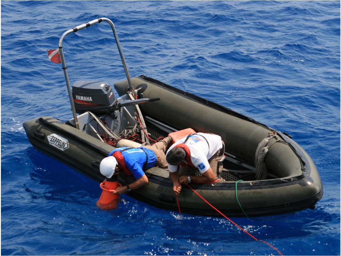
Figure 6.7: The RHIB boat used as a broadband target for passive acoustic localization algorithms. The noise produced by this boat as it moves through the water is recorded by the hydrophones of the hydrophone array moored to the seabed.
