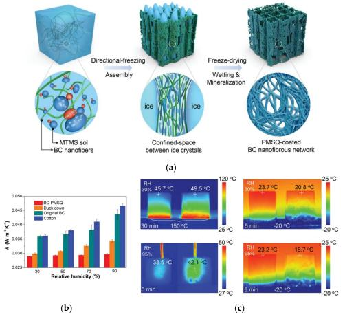
**Figure 6.** Nanoellulosic hybrid aerogels for thermal insulation. (a) Processing principles and synthesis of the BC–PMSQ hybrid aerogels. (b) Thermal conductivities  $\lambda$  of BC–PMSQ, down feathers, and pure BC membranes. (c) Durable thermal insulation performance was evaluated by optical and infrared images. Adapted with permission from Ref. [132], Copyright 2021, Wiley-VCH GmbH.
