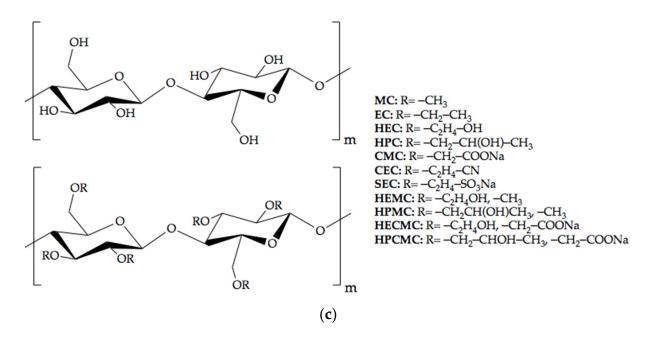
**Figure 2.** Chemical structure of cellulose and its derivatives. (a) Chemical structure of cellulose. (b) Scanning electron micrograph images of *Acetobacter xylinum* and formation of bacterial cellulose. Adapted with permission from Ref. [43] Copyright 2019, Springer Nature. (c) The chemical structure of cellulose and some of its derivatives. Adapted with permission from Ref. [54] Copyright 2016, WILEY-VCH Verlag GmbH & Co. KGaA, Weinheim.
