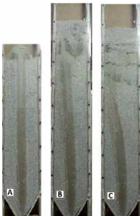
Fig. 14. Half sectional column tests at H : a) external spout and fountain formation at H \approx 0.95 H_m , b) submerged spouting at H \approx 1.05 H_m c) spouting instability with spout wandering at H \approx 1.05 H_m
