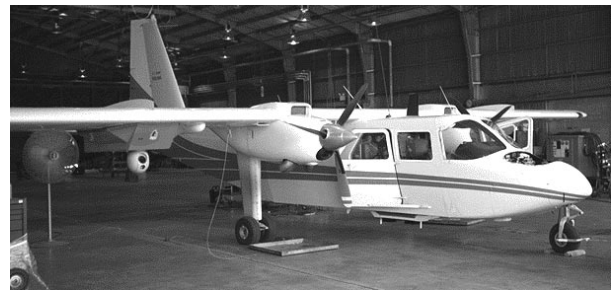
Figure 2: The Night Vision and Electronic Sensors Directorate Islander aircraft. Camera turret is below wing at left.
