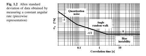
having slope equal to 0 is relevant to angle random walk. This means that the random walk noise is a white noise contribution to the angular velocity estimation. This can be explained observing that the rotation angle can be calculated by integrating the angular rate and, as previously explained, a random walk stochastic process is obtained by integrating a white noise stochastic process.
