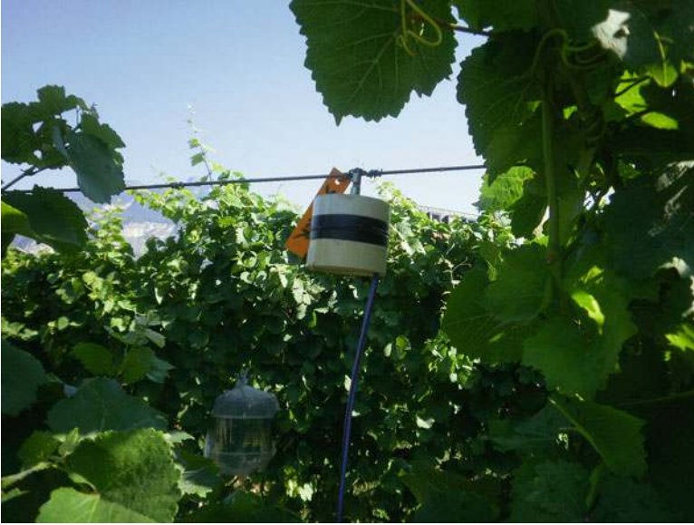
Fig. 9.4 A prototype shaker hung on the trellising wire in the experimental vineyard in San Michele all'Adige. A cage for constraining the animals during field trials is visible in the neighbouring row behind (Photo: J. Polajnar)
