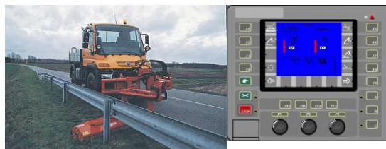
Figure 14. The example vehicle and its display unit as a control desk
