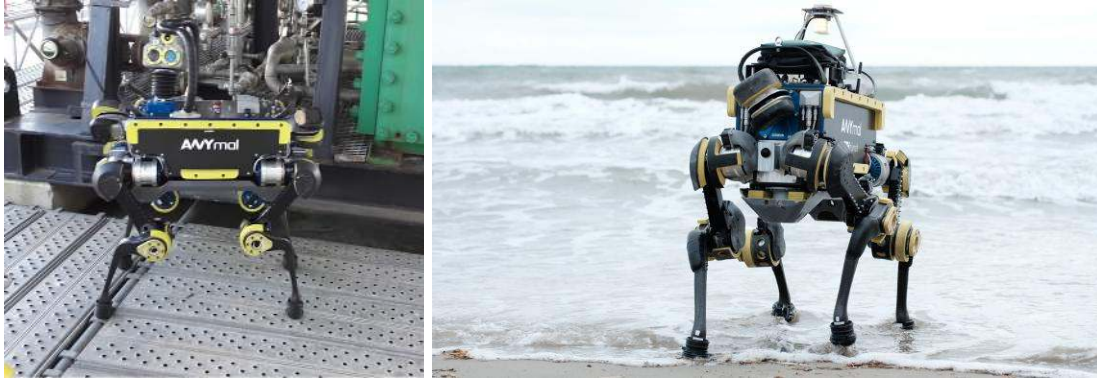
Figure 1: The quadrupedal robot ANYmal can be employed for industrial inspection (left) and search and rescue missions (right) in harsh environments.
