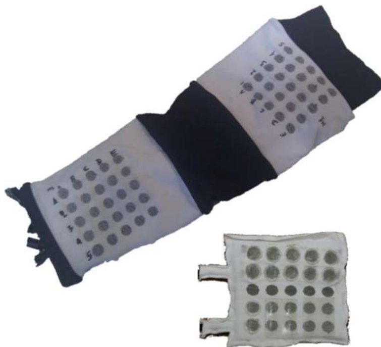
Fig. 2 Two versions of SMARTEX electrode. Single electrode array version right corner and 4-electrode array garment for full upper limb sFES applications
