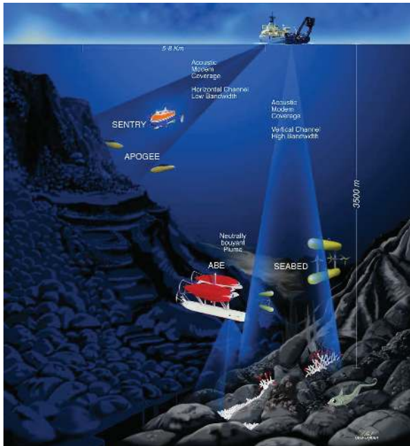
Fig. 1. Acoustic data-packets broadcast from the ship can be used for combined communication and navigation by multiple underwater vehicles. Image credit: Paul Oberlander, WHOI.
