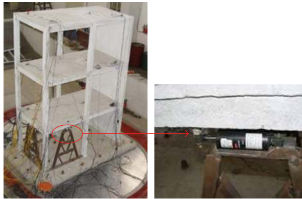
Figure 27: Eccentric vibration control experiment with MR damper.
