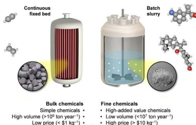
Figure 1. The illustration depicts the strict differences in operation and market between hydrogenation reactions applied in the manufacture of bulk (left) and fine (right) chemicals.
