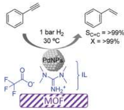
Fig. 9 Semi-hydrogenation of alkynes catalyzed by Pd nanoparticles supported by a metal-organic framework embedded in an ionic liquid microphase.
