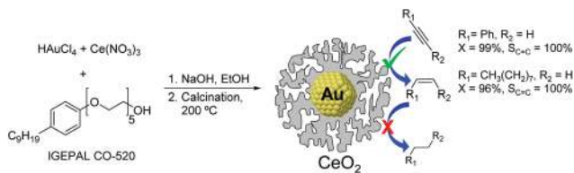
Fig. 18 Preparation of Au@CeO 2 NPs by a simultaneous coprecipitation method and selective hydrogenation of alkynes with prevented over-hydrogenation.
