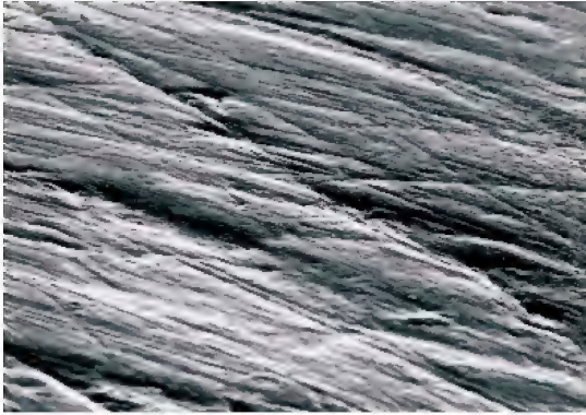
Fig. 7. Cervus canadensis at 500 \times ; an over-scratched surface where new scratches would fall upon preexisting ones.
