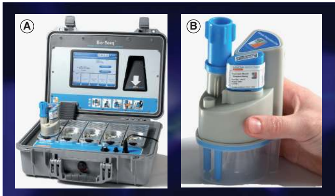
Figure 4. BioSeq Portable Veterinary Diagnostic System. (A) Portable PCR instrument with five independent thermocyclers (running assay in far left thermocycler) with built in communications, including global positioning system, WiFi and Bluetooth technology. (B) Disposable automated sample-preparation unit processes raw sample into PCR mixture allowing test to be conducted at pen-side.
