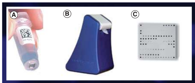
Figure 1. Clondiag Chip technologies ArrayTube® platform. (A) ArrayTube (with probe array chip at the bottom of the tube), (B) the ATR 03 reader (connected to a PC or laptop to run image acquisition and analysis) and (C) magnification of probe array chip. The detection reaction consists of horseradish peroxidase (HRP) and a HRP substrate, tetramethylbenzidine, which react to form a blue precipitate.
