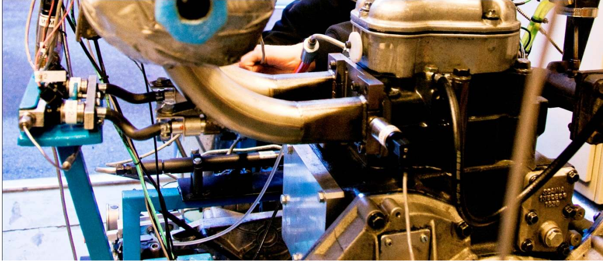
Figure 13 Single cylinder engine used in the experiments, the installation of the gas injectors is visible on the left.
