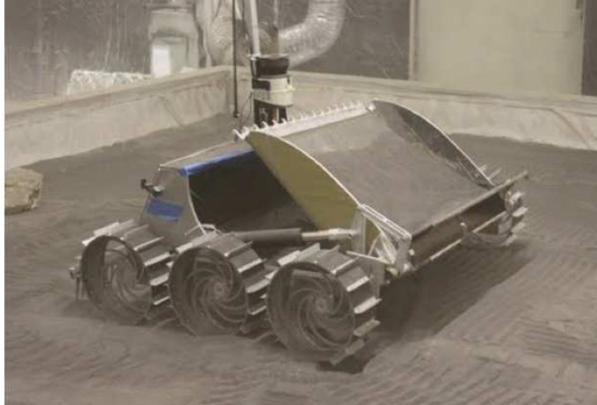
Fig. 2: Lysander, a lightweight scraper excavator, transporting lunar regolith simulant
