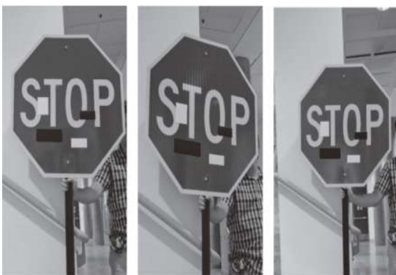
Fig. 5 Attacker puts some stickers on a road sign to confuse an autonomous vehicle's road sign recognizer from any viewpoint (Image credit: Eykholt et al. [20] )
