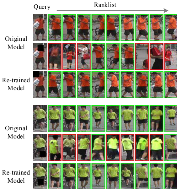
Figure 4: Vulnerability of ReID model to occlusion at test time. The queries are occluded at the position most adversarial to the original or re-trained model, i.e. with lowest mAP score. Images with green and red boundary denote true positive and false positive respectively. The original model fails undesirably when occlusion happens at some positions, which is frequent on the test set. After re-training, the model is much more robust to occlusion. Zoom in to see the black square occlusion masks on four query images.
